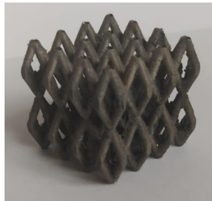
Figure 1. Final Nickel-Phosphorous Microlattice obtained from the production method developed.
