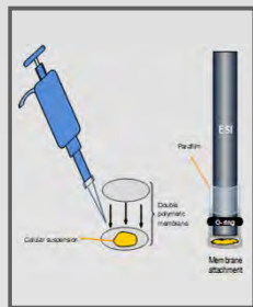
General procedure for whole cells immobilization onto the potentiometric transducer using polymeric membranes
