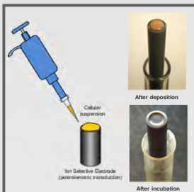
General procedure for whole cells immobilization onto the potentiometric transducer using different material matrices
