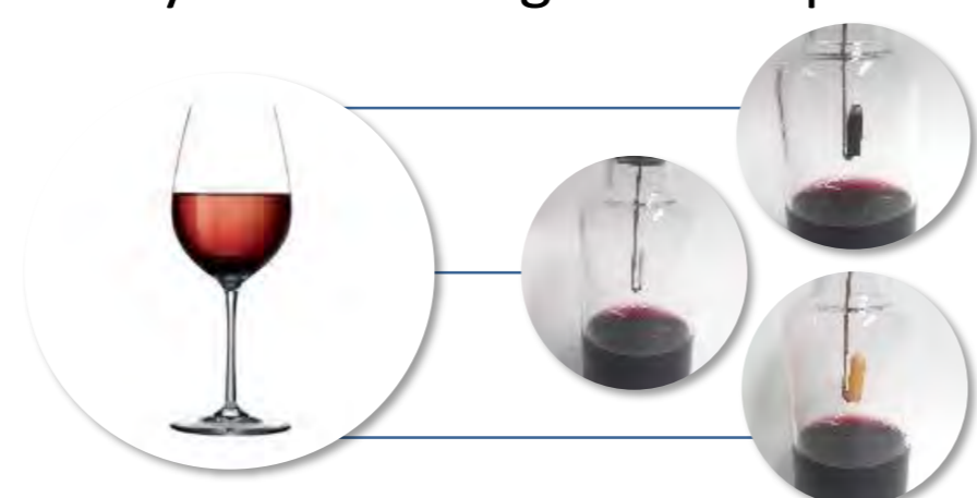
Figure 1: HS-BA \mu E and HS-HF \mu E analysis of the aroma profile in wines samples.
