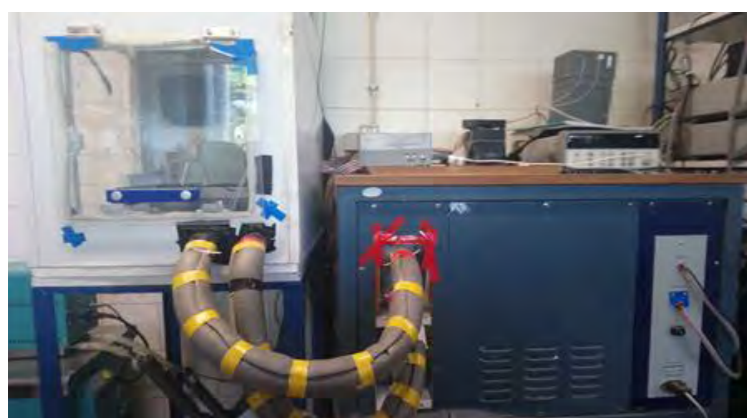
Figure 1. Experimental apparatus consisting of a modified LKB 10700-1 flow calorimeter coupled to cell count, ethanol and CO 2 sensors.
